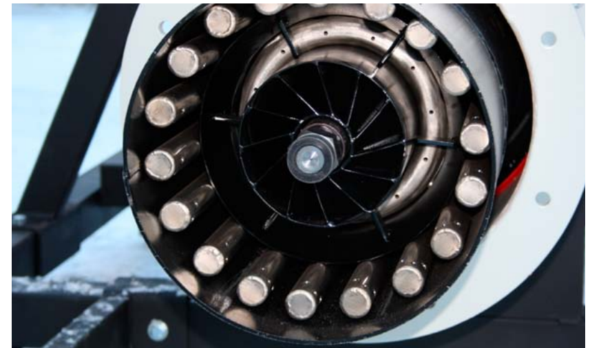
The grinding plant in Vampula has received a new burner, which enables the use of biogas.
